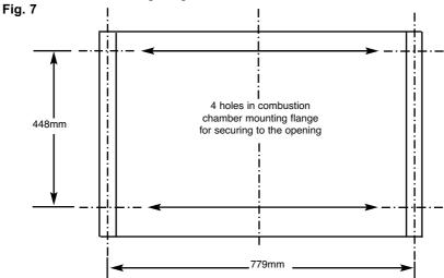
b) DO NOT SECURE THE COMBUSTION INTO THE OPENING AT THIS POINT AS ACCESS WILL STILL BE REQUIRED TO RUN THE GAS SUPPLY PIPEWORK AS DETAILED IN SECTION 2.5
