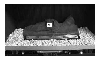
c) Fit Log "B" into position on left hand side of the fuel-bed base log "A" as shown below in Fig. 21, using the groove in Log "A" as a guide for placement.
