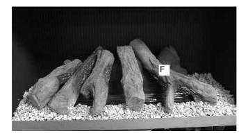
g) Fit Log "G" into position at right hand side of the fuel-bed base log "A" as shown below in Fig. 26, using the raised section in the base log as a guide for position.
