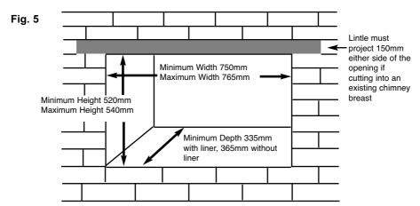
**NOTE**: Please ensure that access holes are cut into either the sides or area above the lintel to allow access to the flue pipe connection if using a flue liner. Such access holes are also advantageous in installations where a flue liner is not required as they provide access for servicing purposes.
