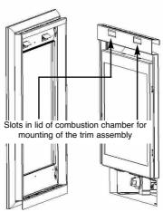
b) The aluminium trim is retained at the base of the firebox by the magnets supplied.
